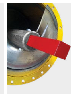
Square One-Bolt Connection
